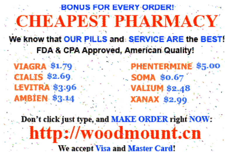
Figure 6.2. An example of image-based spam with noise in order to avoid text recognition using OCR software.
